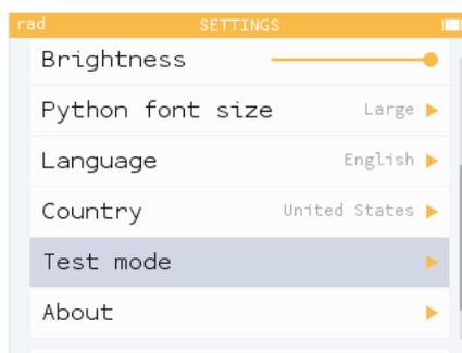
2. Navigate down and press the right arrow or OK to enter **Test mode**.
